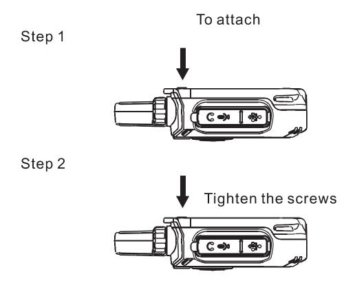
To attach: Place the belt clip as shown in picture & tighten the screws.
